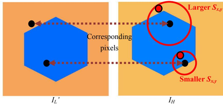
Fig. 12. Local color mapping region  $S_{x,y}$ . Note that the size of  $S_{x,y}$  is inversely proportional to the value of pixel  $(x, y)$  in the iteration map. The black pixels represent the  $I_L^2(x, y)$  and corresponding pixel  $I_H(x, y)$ , while the red pixels represent the pixels found via the local color mapping scheme given Eq. (12).
